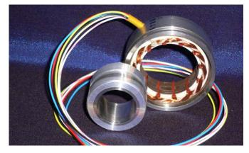
Series RO5032 is a frameless size 21 solid-rotor resolver with a 50mm stator OD and a 32mm airgap diameter. It fits shafts up to 20mm diameter.
