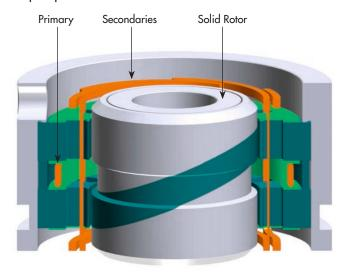
The Rotasyn is similar to a rotary variable differential rotary transformer (RVDT) in which the rotor acts as a magnetic valve completing the flux path. The total flux through the gap is constant—the rotor determines the angular position within the stator bore where the coupling occurs, and thus the relative amplitudes of the output signals.
