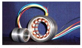
Series RO3620 is a frameless size 15 solid-rotor resolver with a 36mm stator OD and a 20mm airgap diameter. It fits shafts up to 12mm in diameter.
