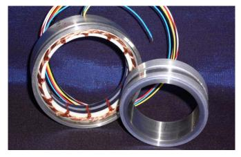
Series RO7557 is a frameless size 30 solid-rotor resolver with a 75mm stator OD and a 57mm airgap diameter. It fits shafts up to 47mm in diameter.
