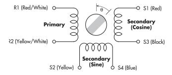
$V_{(S1-S3)} = V_{(R1-R2)} \times TR \times \cos(\theta)$
