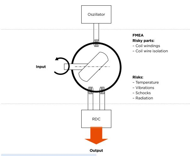
Before and during flight **all** coil windings can be checked
